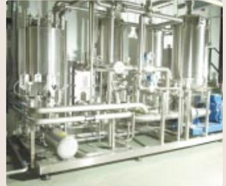
Fig. 9 - A Filtrix CERinox ceramic crossflow filter. The photo shows a 3 module plant, with each module of 40m<sup>2</sup> capable of handling up to 18 hl/hr of yeast slurry – photo supplied by Filtrix AG.
