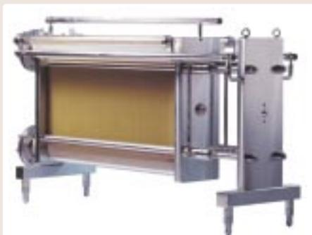
Figure 11: A DSS M39-H Alfa Laval plate & frame polymer membrane crossflow filter capable of handling 35 hl/hr yeast slurry –photo supplied by Alfa Laval Ltd.
