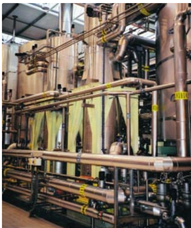
Figure 8: The Symphony external wort boiling system – supplied by Briggs of Burton.
