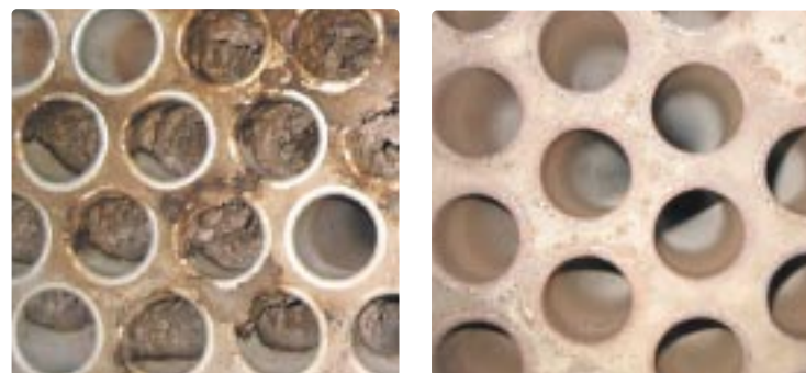
FAR LEFT: Figure 12: The tubes of a conventional internal wort heater after 8 brews.
